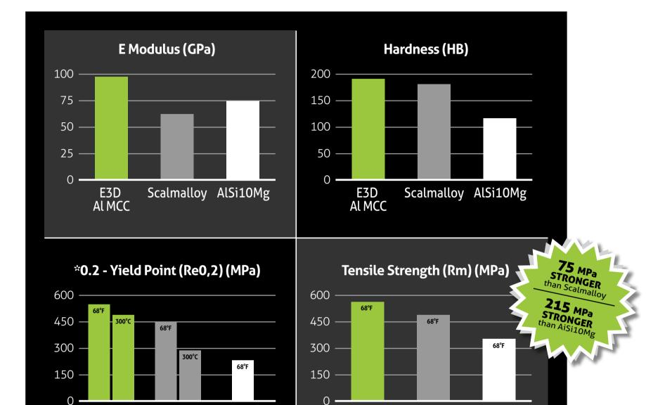
\*At a temperature of 300°F, Scalmalloy lost 36% of its yield strength (450 down to 290 MPa) while the Elementum 3D (E3D) AlMMC only lost 12% of its considerably higher yield strength (552 to 485MPa). At 300°F the E3D AlMMC still has higher strength than scalmalloy at room temperature by a significant margin. Data source: anonymous automotive company.
