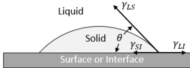
Figure 3: Simplified schematic of a flat heterogeneous nucleation site. Solid surfaces within a melt that can act as a heterogeneous nucleation site include impurities, inoculant particles, mold walls, etc. Adapted from Reed [2].
