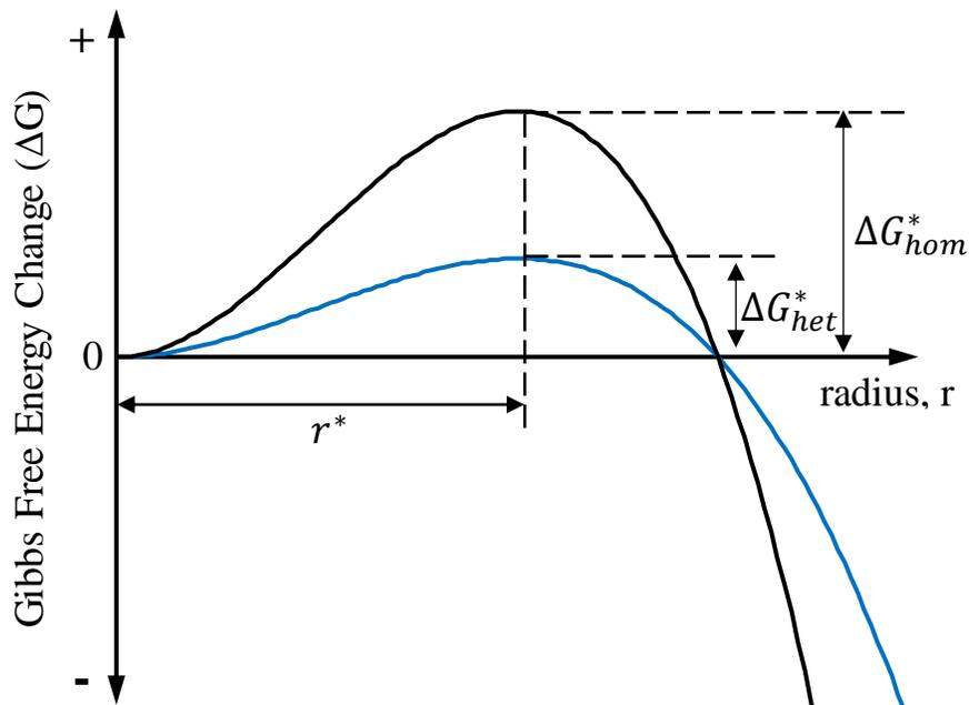
Figure 4: Gibbs free energies of homogeneous and heterogeneous nucleation. Notice the critical radii are equal while the heterogeneous nucleation requires less energy to nucleate a grain.
