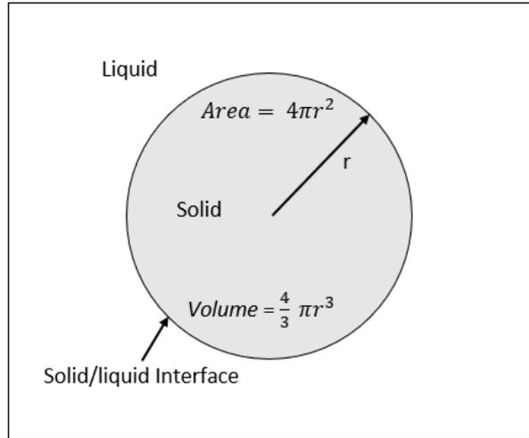
Figure 1: Annotated schematic of a homogeneously nucleated particle. Adapted from Callister [1].
