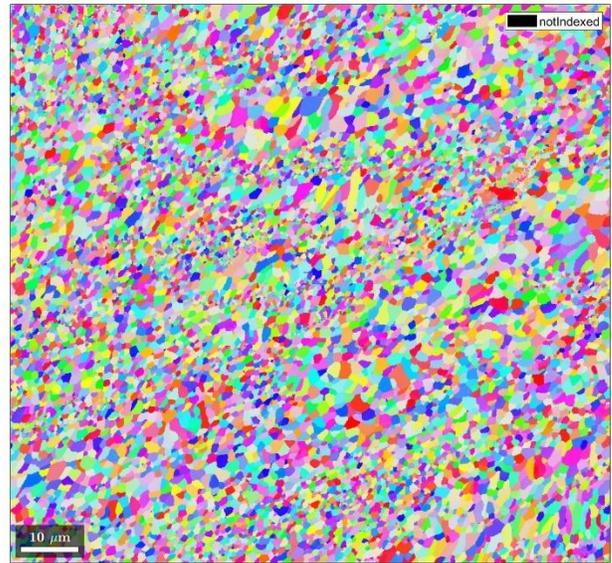
Figure 7: Elementum 3D’s A6061-RAM2, processed by L-PBF, employs inoculants for grain nucleation shows a dispersion of fine grains (average size 1 – 2 μm) that prevent hot tearing and minimize porosity. (Image courtesy of Ethan Sullivan, Colorado School of Mines)
