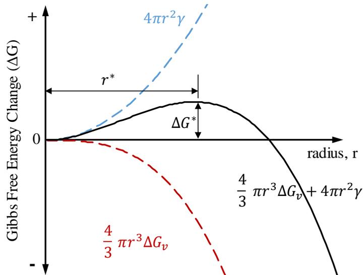
Figure 2: The individual components of Eq.1 and the summation of the two components are plotted. The summation curve clearly displays the conceptual activation free energy ( $\Delta G^*$ ) and the critical radius ( $r^*$ ). Adapted from Callister [1].
