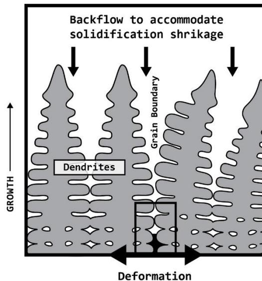
Figure 5: Schematic of primary dendrite formation, which leaves the regions between dendrites free for the remaining liquid in the system to fill. As the material cools the shrinkage produces deformation and stresses that can result in hot tearing. Adapted from Rappaz, et al. [3].
