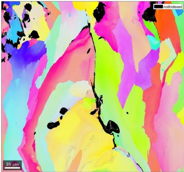
Figure 6: EBSD image of traditional AA6061, processed by L-PBF. The alloy solidifies with large columnar grains that result in clear examples of hot tearing and a poor grain structure that is unsuitable for structural application. (Image courtesy of Ethan Sullivan, Colorado School of Mines)
